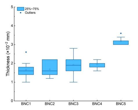
**Figure 2.** Thickness of BNC membranes cultivated from *K. medellinensis* (ID13488) for 10 days, after alkaline treatments with different exposure times and after autoclave treatment.: NaOH, short exposure (BNC1); NaOH, long exposure (BNC2); KOH, short exposure (BNC3); KOH, long exposure (BNC3); autoclave (BNC5).
