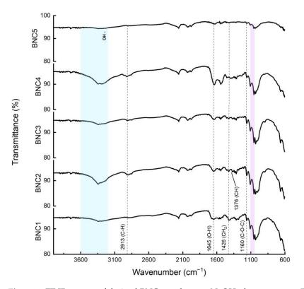
**Figure 4.** FT-IR spectra of derived BNC membranes: NaOH, short exposure (BNC1); NaOH, long exposure (BNC2); KOH, short exposure (BNC3); KOH, long exposure (BNC4); autoclave (BNC5), antisymmetric out-of-phase bending in purple and hydroxyl functional groups in blue.
