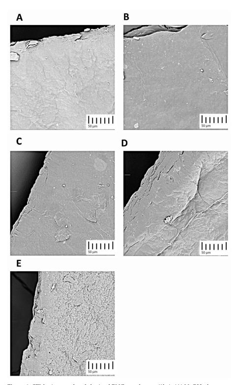
**Figure 3.** SEM micrographs of obtained BNC membranes (1kx): **(A)** NaOH, short exposure (BNC1); **(B)** NaOH, long exposure (BNC2); **(C)** KOH, short exposure (BNC3); **(D)** KOH, long exposure (BNC3); **(E)** autoclave (BNC5).
